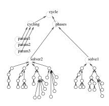
Figure 11: Grafting operation for a CHT coupling setup: a CFD solver coupled with a thermal solver
