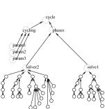
Figure 6: Grafting operation for a coupling setup: a CFD solver coupled with a thermal solver
