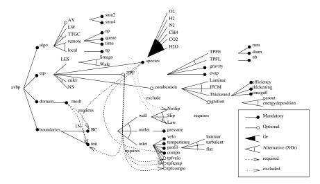
Figure 8: Feature Diagram of the CFD LES code AVBP  $6.2\beta$  using the notation of Kang [7]. The diagram is simplified: more than sixty boundary conditions are available, and only the major model parameters are shown.
