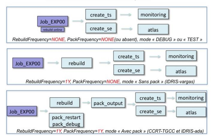
The diagram below details the added jobs pack\_debug, pack\_restart and pack\_output as well as the directories those jobs are using. Note that the files are temporarily stored in the \$WORKDIR/IGCM\_OUT directories before being grouped and sent on Gaya in the IGCM\_OUT directories.
