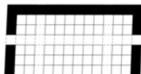
**North fold boundary with a T-point pivot (in\_perio=3)** first row, and first and last columns are closed.
