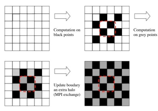
Fig II-3 : SOR solver with extra outer halo
