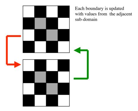
Fig II-2 : boundary update with MPI exchange
